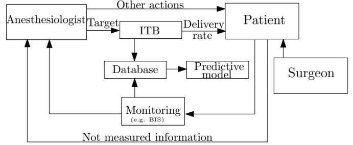
Figure 3: The ITB software and the anesthesia procedure. ITB accomplishes two main tasks: (i) servo-control of the drugs' delivery rate on the basis of the targets fixed by the anesthetist and (ii) monitoring and storing the patient's signals and the anesthetist's actions in a database.
