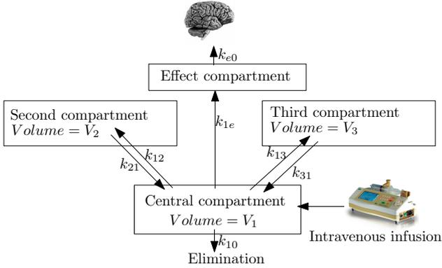
Figure 2: Compartment modeling seeks to estimate the contraction evolution with time of a drug in an effect site (e.g. the brain). The values of the transfer rates ( $k_{10}, k_{21}, k_{12}, k_{31}, \dots$ ) and volumes ( $V_1, V_2, V_3$ ) are defined by the model.
