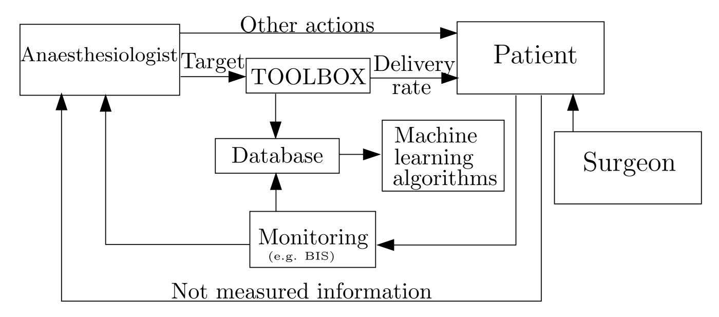
The proposed controller possesses adaptive control features and relies on the availability of several input signals measuring the patient condition and the operation state.
